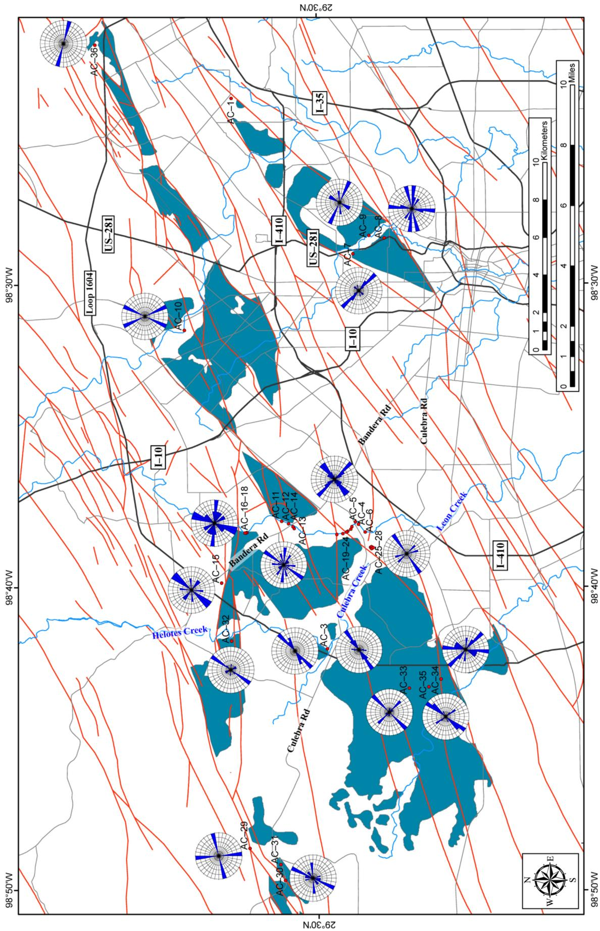
Figure 4. Map with Austin Chalk outcrop (blue shaded area), mapped fault traces (red lines) from the Geologic Map of Texas (Bureau of Economic Geology, 1992), and rose diagrams for extension fractures in this study area.
