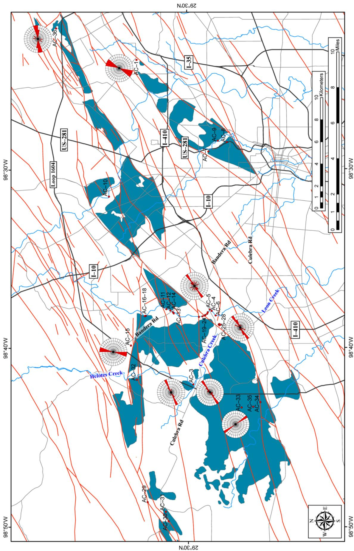
Figure 5. Map with Austin Chalk outcrop (blue shaded area), mapped fault traces (red lines) from the Geologic Map of Texas (Bureau of Economic Geology, 1992), and rose diagrams for faults measured in outcrops within the study area.
